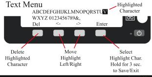
Enter – pressing enter momentarily adds the character to the current text string on the display. Press and hold enter for approximately 3 seconds to save and exit the text writer.
